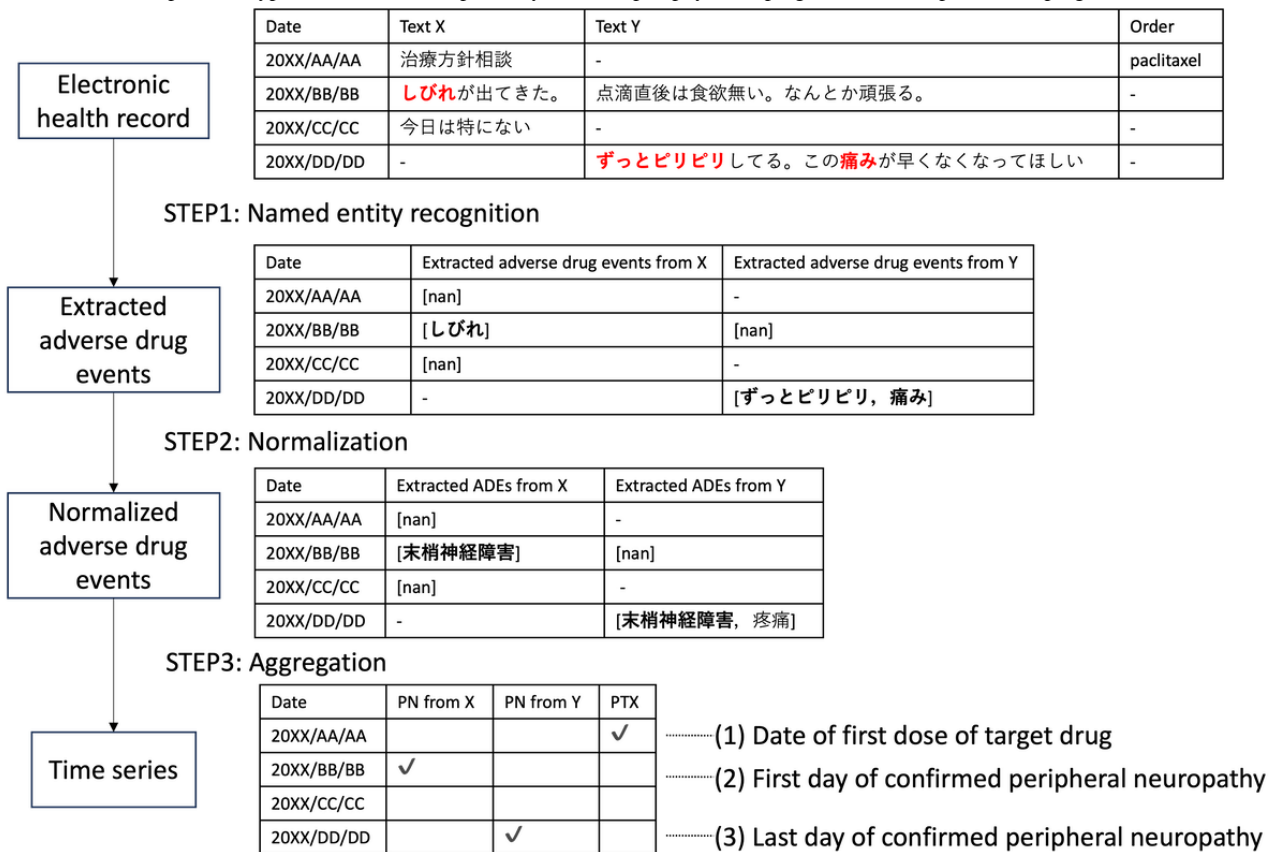
Figure 3. Workflow of our natural language processing system, which is composed of named entity recognition, normalization, and aggregation. Text X and Text Y are examples of 2 types of documents respectively, for example, physician progress notes and pharmacist progress notes.
