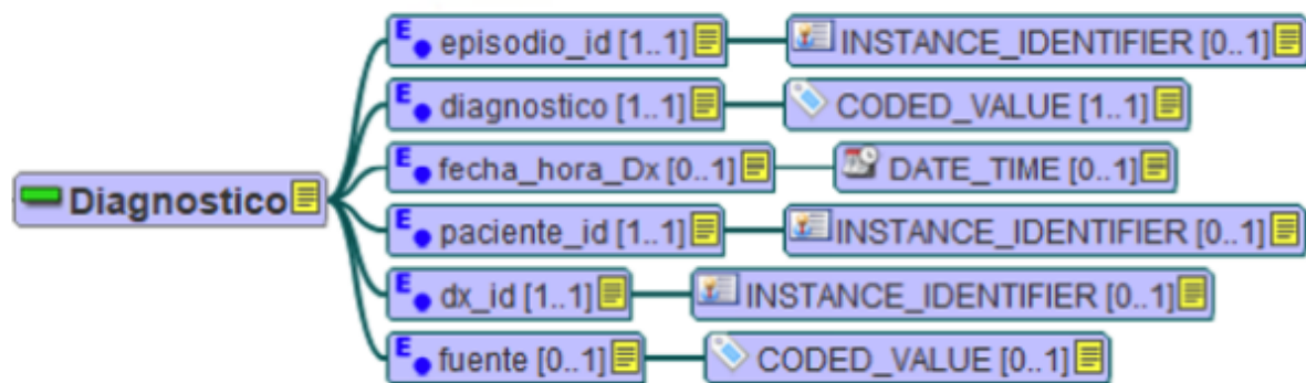
Figure 1. Mind map of the EN/ISO 13606 “diagnosis” archetype in Spanish, modeled with LinkEHR. The “diagnosis” entry has 6 elements: episode_id, diagnosis, diagnosis_datetime, patient_id, diagnosis_id, and source. Each of them has its corresponding data type. EN/ISO: European Norm/International Organization for Standardization.
