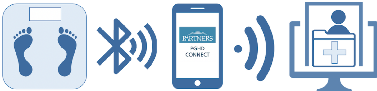
Figure 1. Flow of weight information. Weight data are collected from the Bluetooth-connected scale, transmitted via a Bluetooth connection to the PGHDConnect app, and then via the internet to the electronic medical record.
